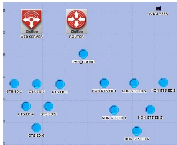
Fig. 2: Variant of 802.15.4 - With and Without GTS
