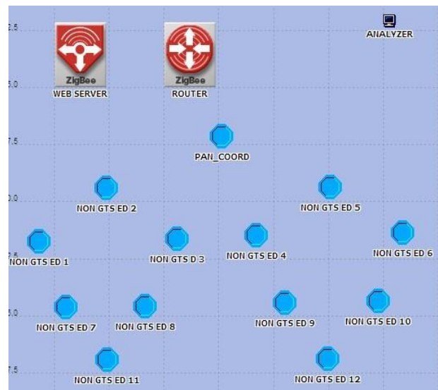
Fig. 3: Variant of 802.15.4 - Without GTS
