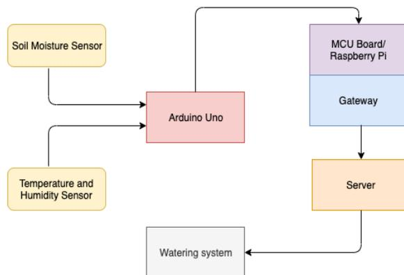
Fig. 1: Setup of the system
