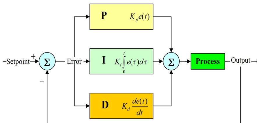
Fig. 3: Outline of the PID controller and formula
