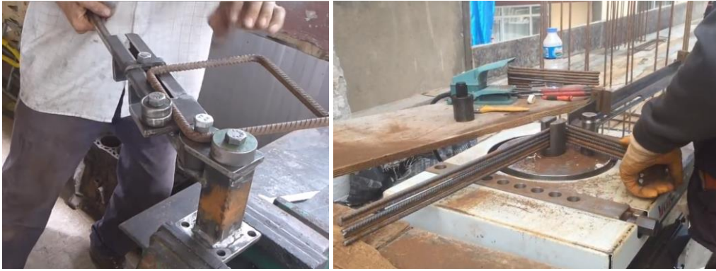
Fig. 2: Examples of bending process (a) Manual bending process, (b) Semi-automatic bending machines
