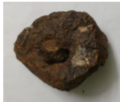
Fig. 11: Magnetite (Earth Rock). Cratering features not observed on their surface
