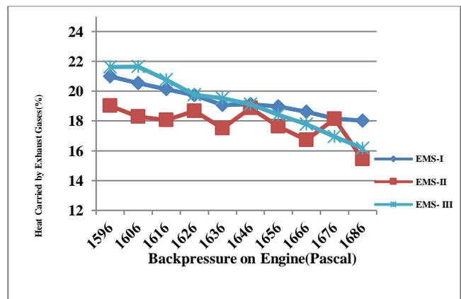
Fig. 4: Variation in heat carried away by exhaust gases in percentage vs. backpressure on the engine for different load conditions using Exhaust Manifold Systems
