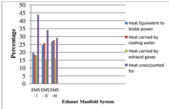
Fig. 6: Heat balance sheet for Exhaust Manifold Systems at constant load 5 Kg
