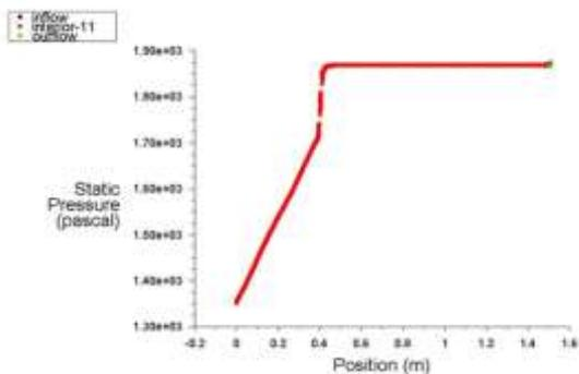
Fig. 9: Variation in backpressure on the engine during the flow through EMS - II at constant Load 5 Kg.
