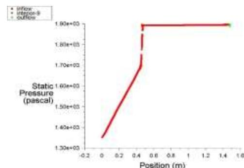
Fig. 10: Variation in backpressure on engine during the flow-through EMS - III at constant Load 5 Kg.
