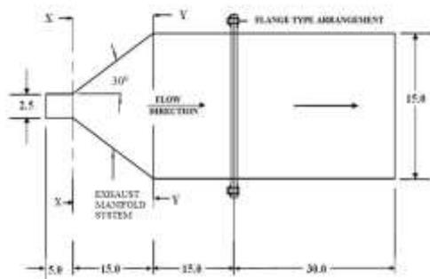
Fig. 1: Exhaust Manifold System
