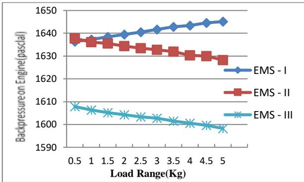
Fig. 5: Variation in backpressure on the engine during experimentation vs. different load conditions for Exhaust Manifold Systems
