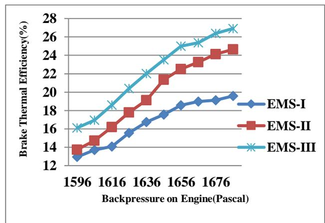
Fig. 3: Variation in brake thermal efficiencies vs. backpressure on the engine for different load conditions using Exhaust Manifold Systems
