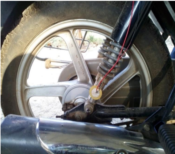
Fig. 2: To mount the sensor in the shock absorber
