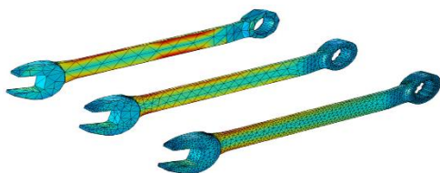
Fig. 15: Starting with a very rough mesh, the first few iterations of the mesh refinement study of the wrench
