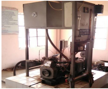
Fig. 3: 4-stroke single cylinder diesel engine
