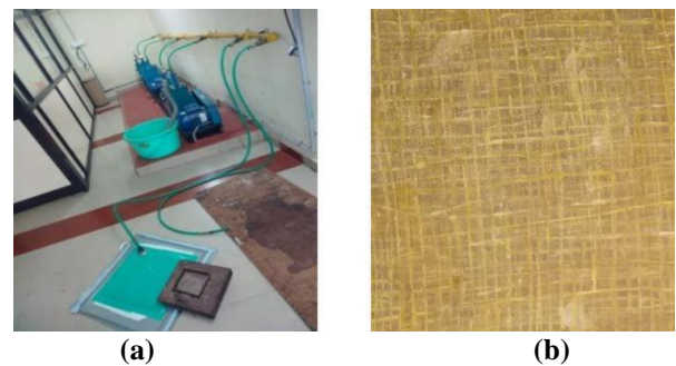
Fig. 2: (a) Vacuum bagging method, (b) Prepared composite
