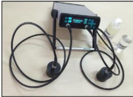
Fig. 7: Portable ultrasonic non-destructive indicating tester
