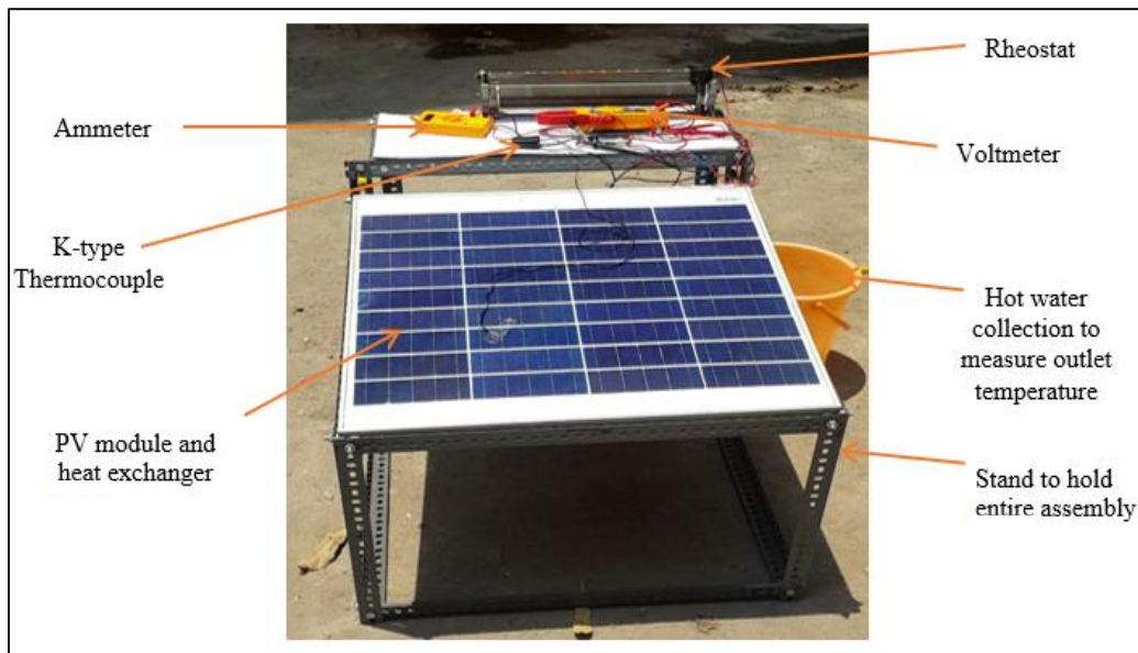
Fig. 6: Hybrid PV/T solar water system with measuring instruments
