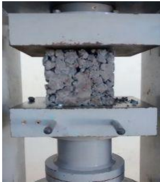
Fig. 1: Cube under compression test
