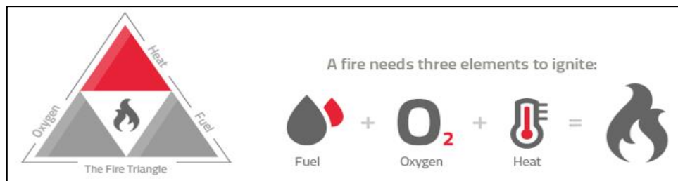
Fig. 3: Fire triangle and elements of fire
