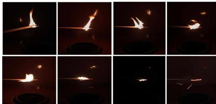
Fig. 10: Solid based fuel flame extinguishing
