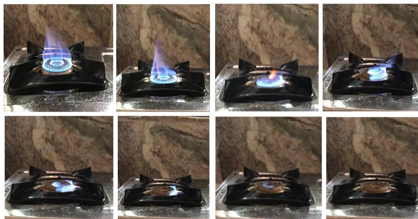
Fig. 9: Sequence of images of gas fire leading to extinction
