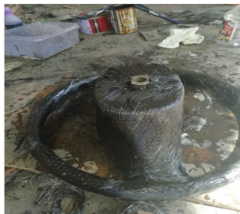
Fig. 1: Steering wheel by Hand lay-up technique
