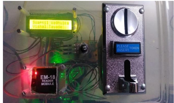
Fig. 6: Coin acceptor in the vending machine
