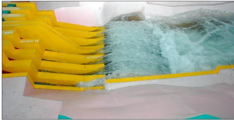
Fig. 4: Performance of ski jump bucket ( Q=11500 \text{ m}^3/\text{s} , RWL El. 1192 m)
