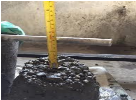
Fig. 2: Slump measurement of EPS concrete
