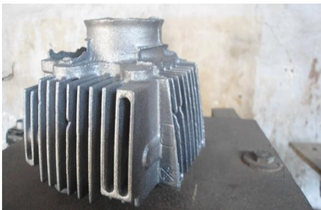
Fig. 2: Cold defect in HH block
