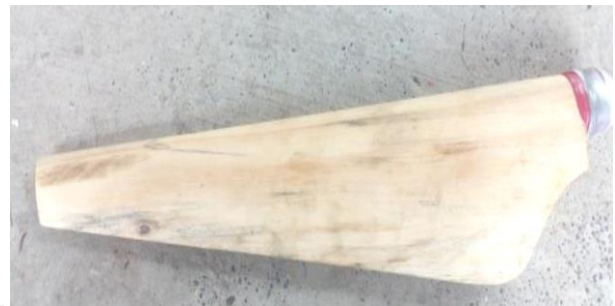
Fig. 3: NACA 63(2)215 Airfoil blade-Actual
