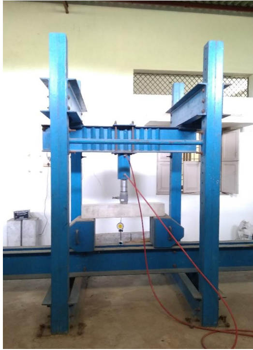
Fig. 3: Loading frame experimental analysis
