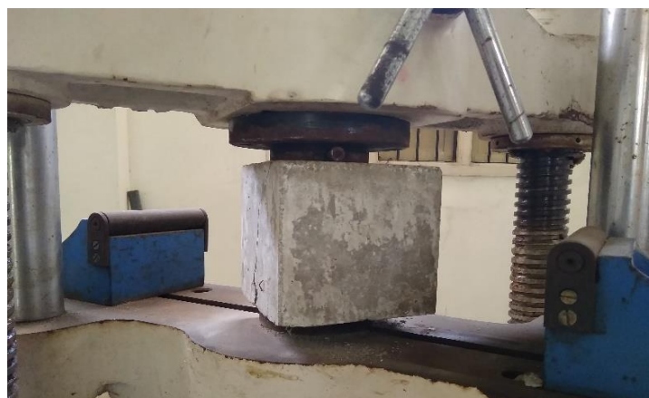
Fig. 2: Cube testing work progress
