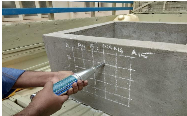
Fig. 5: Rebound hammer test
