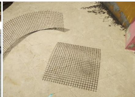
(b) Fig. 4: (b) Welded wire mesh
