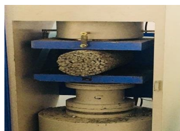
Fig. 3: Split Tensile test on specimen
