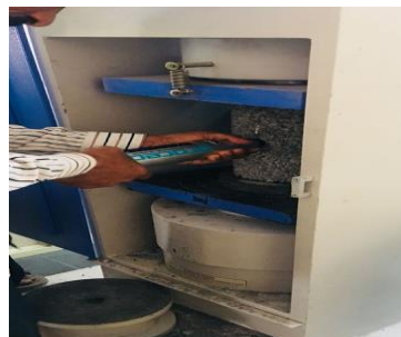
Fig. 2: Rebound hammer test on a specimen
