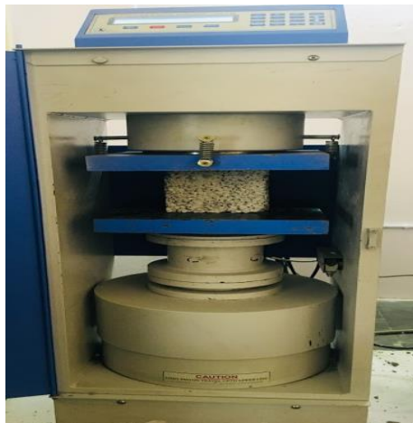
Fig. 4: Compression test on a specimen
