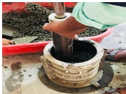
Fig. 1: Compaction with standard proctor rammer
