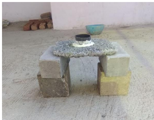
Fig. 5: Infiltration rate test setup
