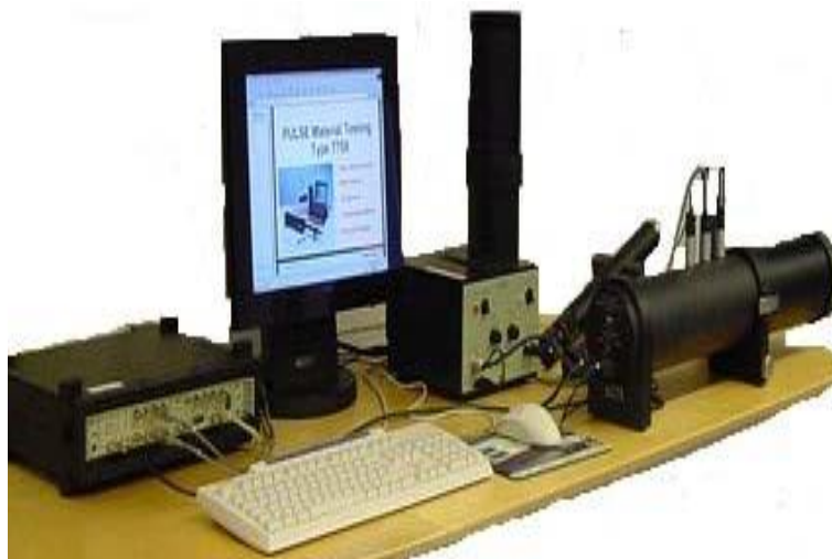
Fig. 4: Experiment of Impedance Tube
