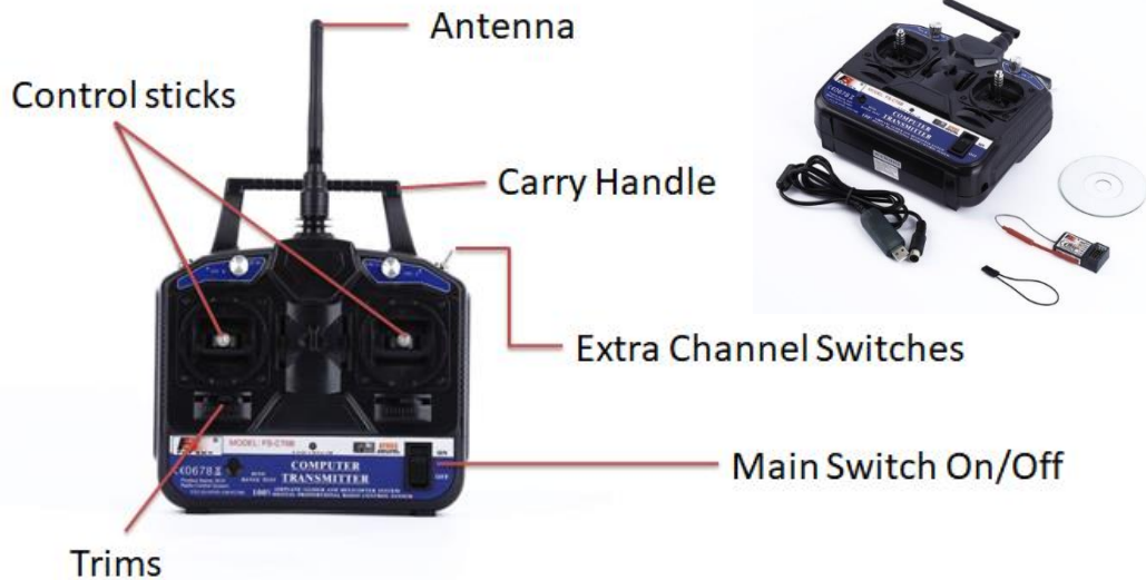
Fig. 2.17: Radio Controller (Transmitter and Receiver)[9]
