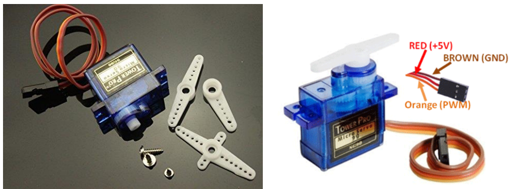
Fig. 2.19: Servo Motor and Pinouts (Wires) [10]
