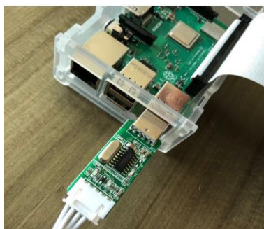
Fig. 4: Hardware integration of Nova PM sensor SDS011 with Raspberry Pi 3B
