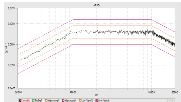
Fig. 7: Random Vibration test plot for the 3 rd -row profile of ECU
