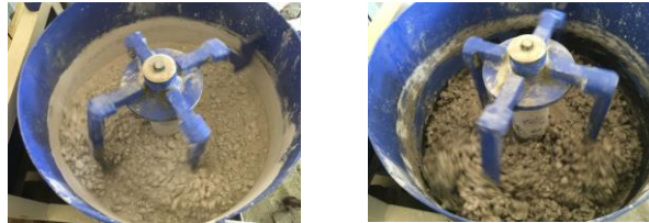
Fig. 2: Dry mix and Wet mix in the pan mixer
