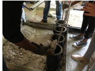
Fig. 3: Compaction by tamping rod
