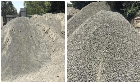
Fig. 1: C rushed sand on site
