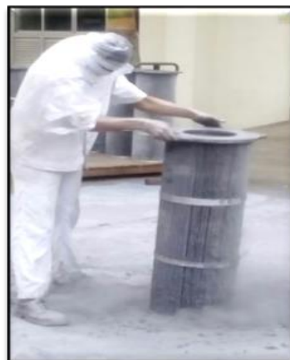
Fig. 1: Traditional manual cleaning of filter [1]
