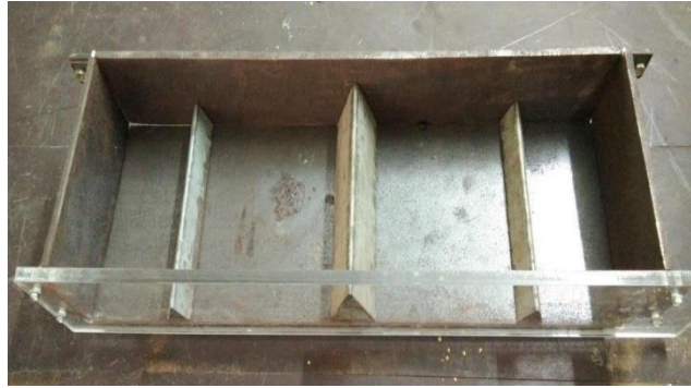
Fig. 4: ASTM C 1579 mould fabricated
