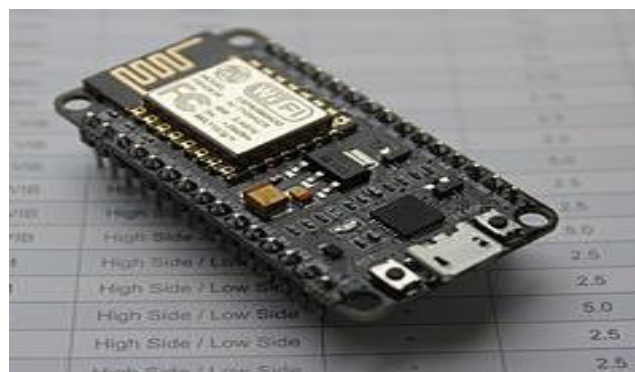
Fig. 3: Node MCU connected to the power supply
