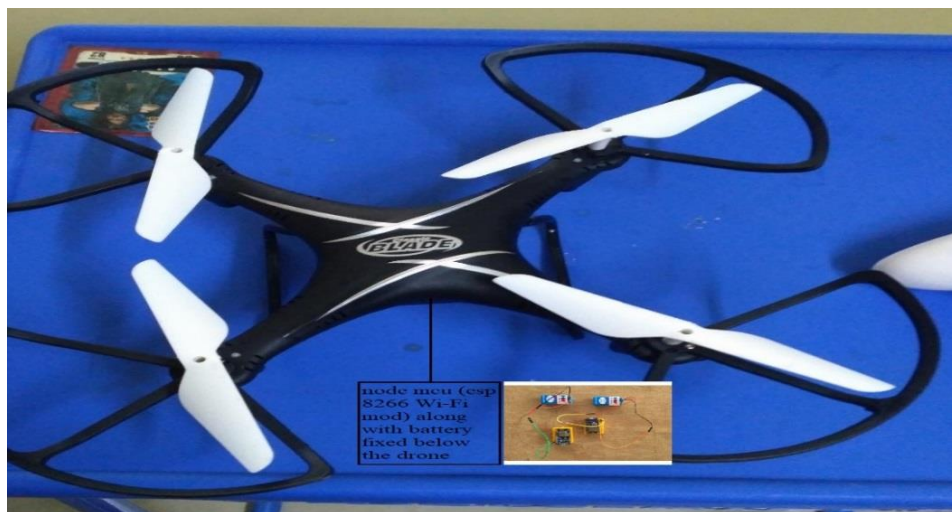
Fig. 5: Implemented drone with a wireless mesh network
