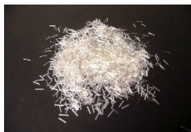
Fig. 1: Glass Fibre (Length 36 mm –as per IRC 15 – 2011)
