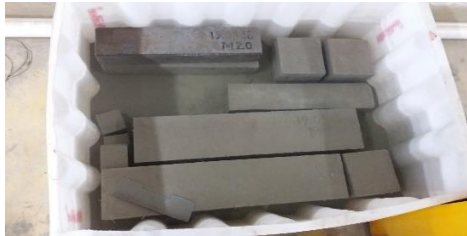
Fig. 11: Concrete curing procedure
