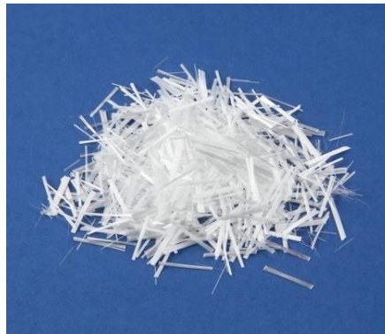
Fig. 3: Glass Fibre (Length = 36 mm), (as per IRC: 15 – 2011)
