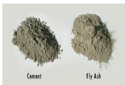
Fig. 2: Fly ash vs. Cement
