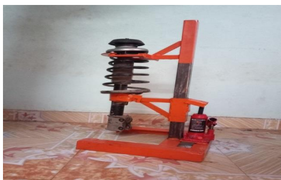
Fig. 2: Working of coil spring compressor
