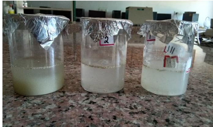
Fig. 5: Settling process of Sample 1, 2, and 3 after the inoculation of M.oleifera seed extract.
