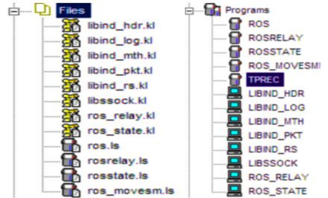
Fig. 11: Fanuc driver files, imported and compiled, in Roboguide
