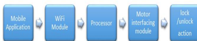
Fig. 2: Block diagram of the child lock control system
