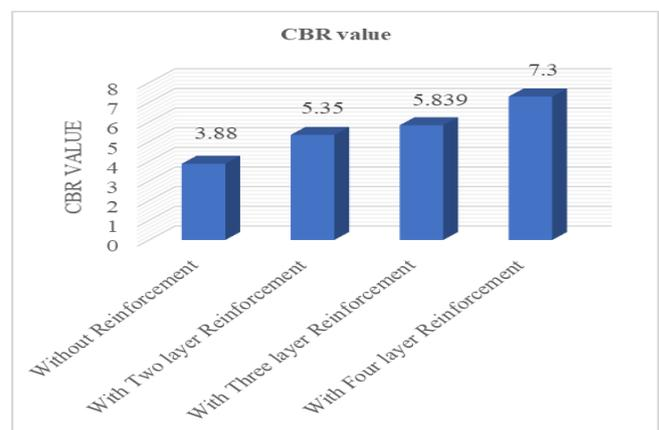
Fig. 10: Comparison graph for CBR test
