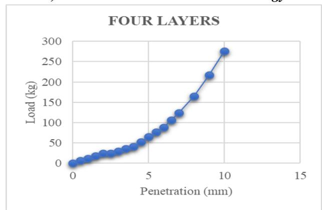
Fig. 8: CBR graph for four layers reinforced soil
