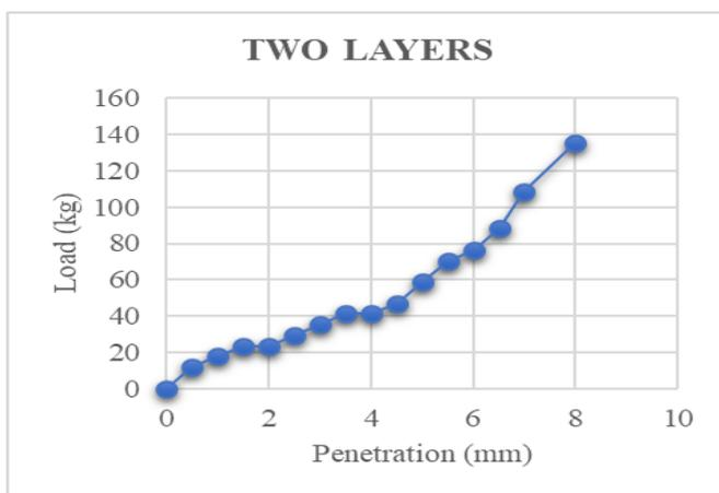
Fig. 6: CBR graph for two layers reinforced soil
