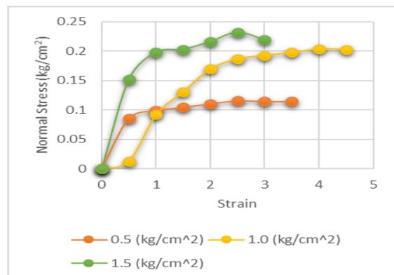
**Fig. 4: Direct shear test results for shear strength of the clayey sand with reinforcement**
