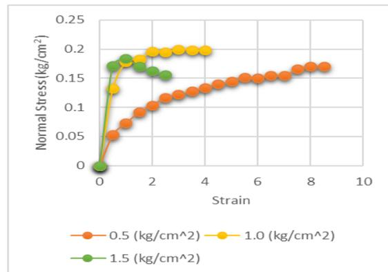
**Fig. 3: Direct shear test results for shear strength of the clayey sand non-reinforcement**
