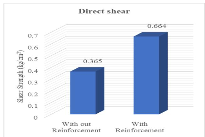
Fig. 9: Comparison graphs for direct shear test
