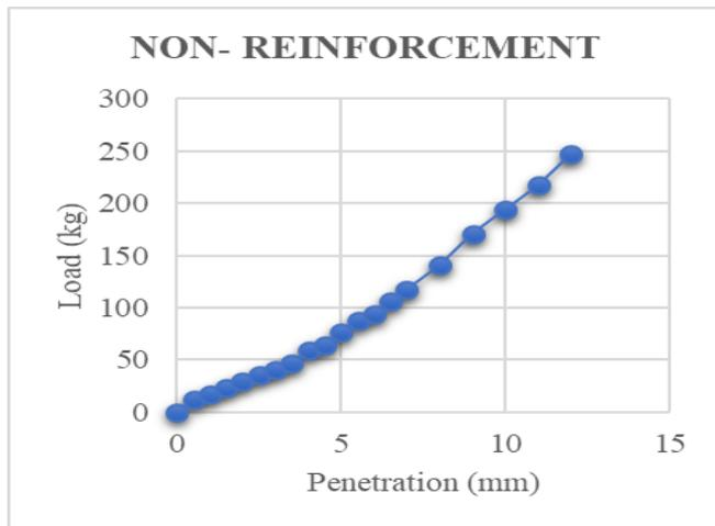
Fig. 5: CBR graph for non-reinforced soil
