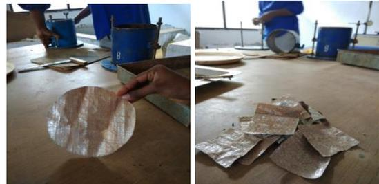
**Fig. 2: Reinforcement Used in CBR and Direct Shear**
