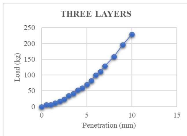
Fig. 7: CBR graph for three-layer reinforced soil
