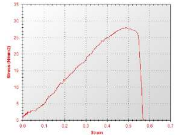
Fig. 10: Tensile test with 10/% composition
