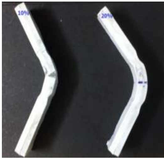
Fig. 4: Specimen after bend test
