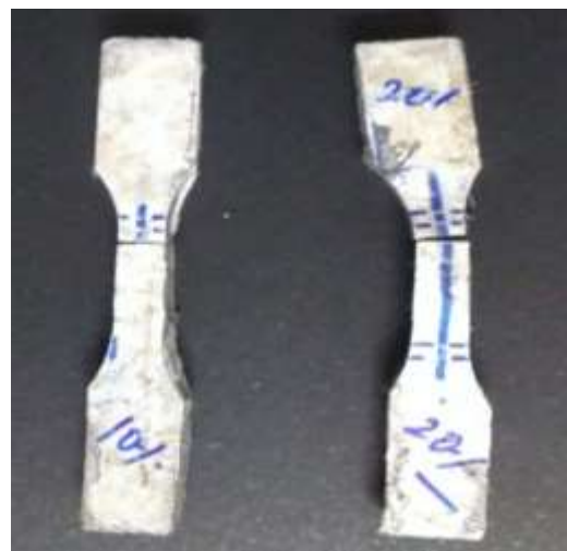
Fig. 7: Specimen after tensile test
