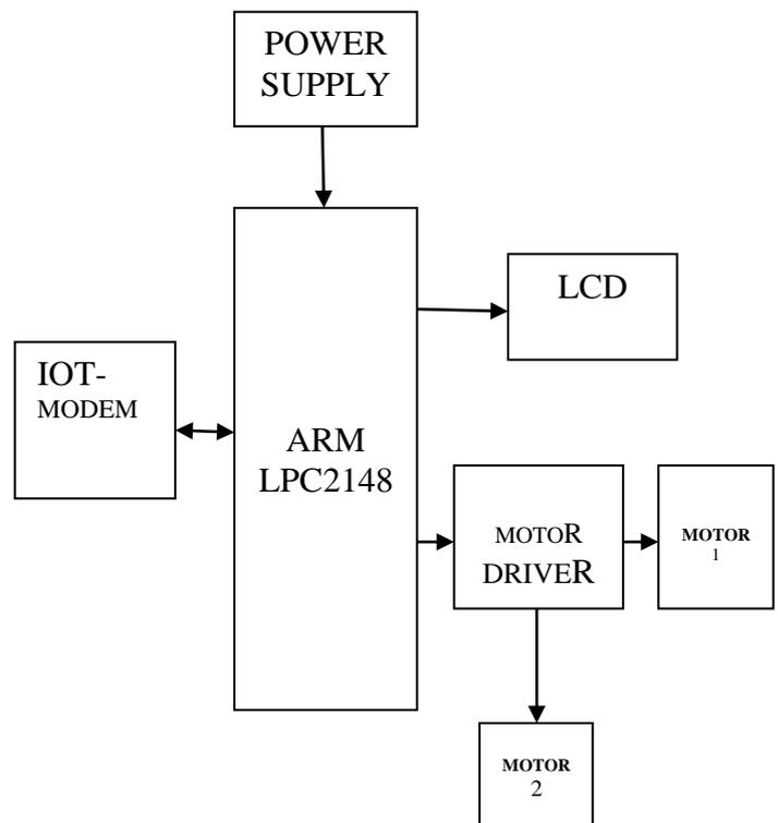
**Fig. 1: Block diagram of the proposed system**
