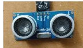
Fig. 3: Ultrasonic Sensor Module
