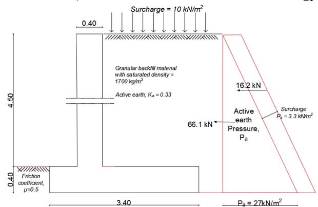
Fig. 7: A case study of retaining wall
