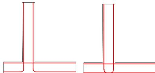
**Fig. 2: Typical reinforcement layout**
