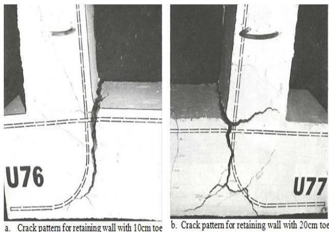
Fig. 5: Crack pattern in retaining wall
