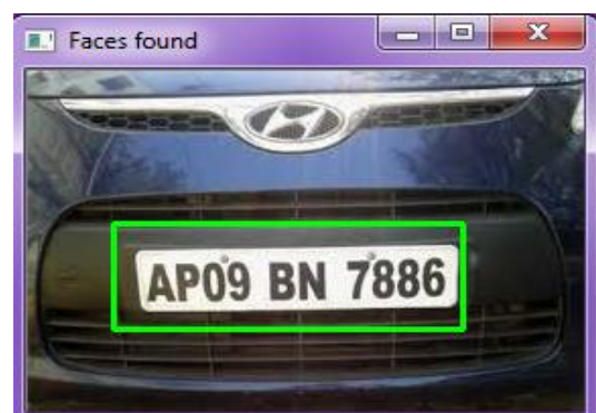
Fig. 5: License plate detection by Haar-cascade
