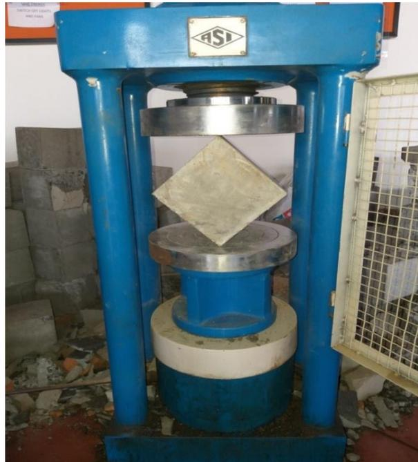
Fig. 4: Split tensile strength test
