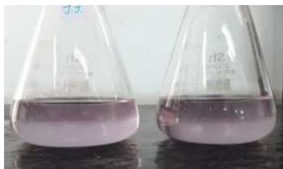
Fig. 6: Effluent before treatment with immobilised beads
