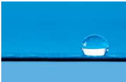
Fig. 10: The angle of contact of water on the surface is what determined the wetting of a surface. If a paint can increase the angle of contact to greater than 90^\circ it can drastically reduce the wetted surface area of the hull.
