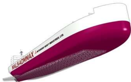
Fig. 1: A diagrammatic representation of the Mitsubishi air bubble injection system. The bubbles form a layer trailing behind till the stern increasing in size. Note that the bottom and sides are void of air lubricant here
