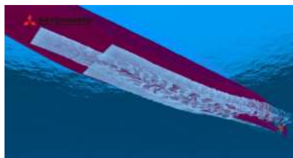
Fig. 4: This depicts the air film lubrication system by Mitsubishi heavy industries LTD. where a film is expelled out in a slit type air release system. Note turbulence induced in the later stages of the film stream
