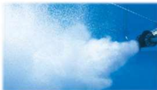
Fig. 3: This shows the air release unit on a test system. A mesh strainer attached to the nozzle, preventing marine growth can be operated in back flush, depending on differential pressures
