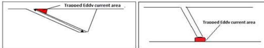
Fig. 10: Left: a Trapped area for less slot angle (30° and 45°); Right: a trapped area for more slot angle (60° and 90°)
