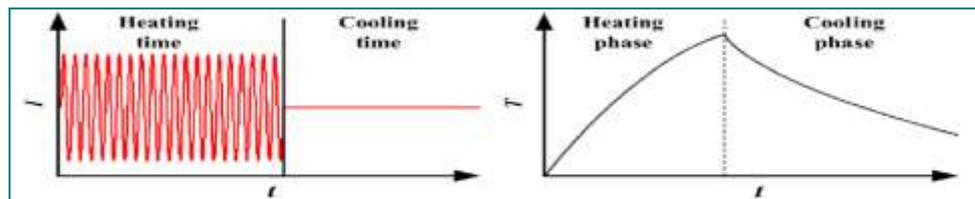
**Fig. 8: Left: Excitation signal, Right: temperature response**
