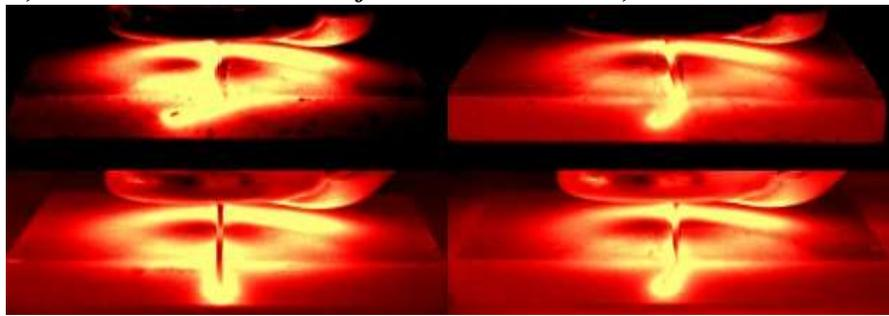
Fig. 9: Thermograms taken at 300ms: (Clockwise) 1: For 30° slot angle; 2: For 45° slot angle; 3: For 60° slot angle; For 90° slot angle
