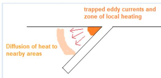
**Fig. 19: Diffusion of heating from localized heating zone to neighbouring area**
