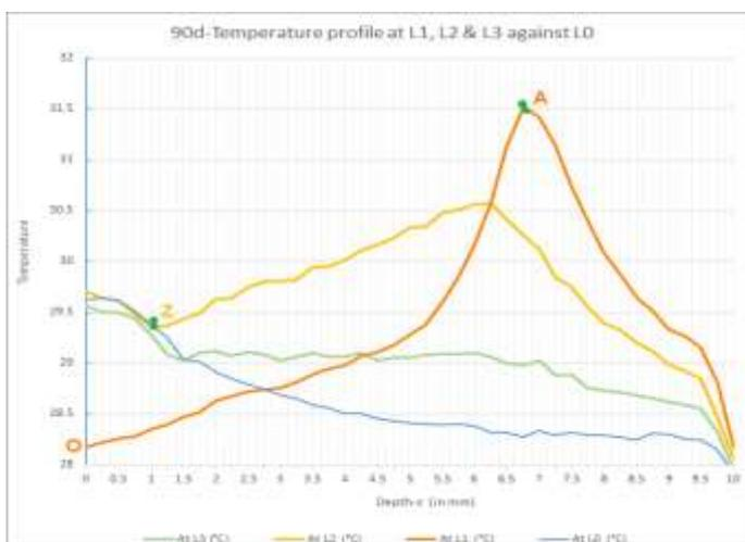
**Fig. 20: Temperature profile along Line L1, L2 & L3 against L0 - 90° slot angle**
