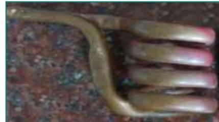
**Fig. 5: Induction coil used in the experiment**
