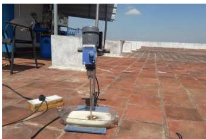
Fig. 3: Experimental Setup for Solar Photo Fenton Treatment
