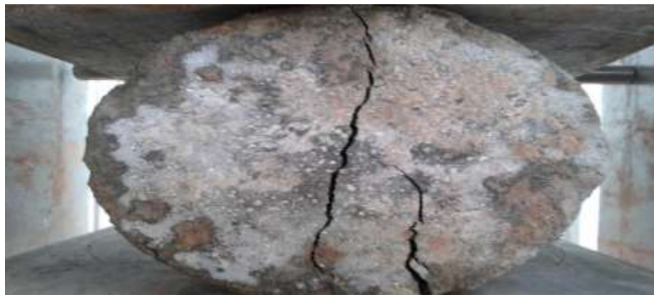
Fig. 6: Split tensile test failure
