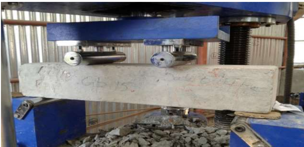
Fig. 5: Flexure strength test set up
