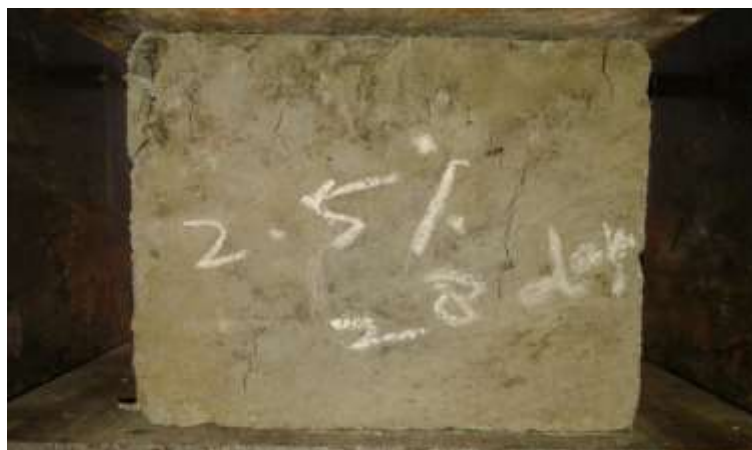
Fig. 1: Cube after compression failure
