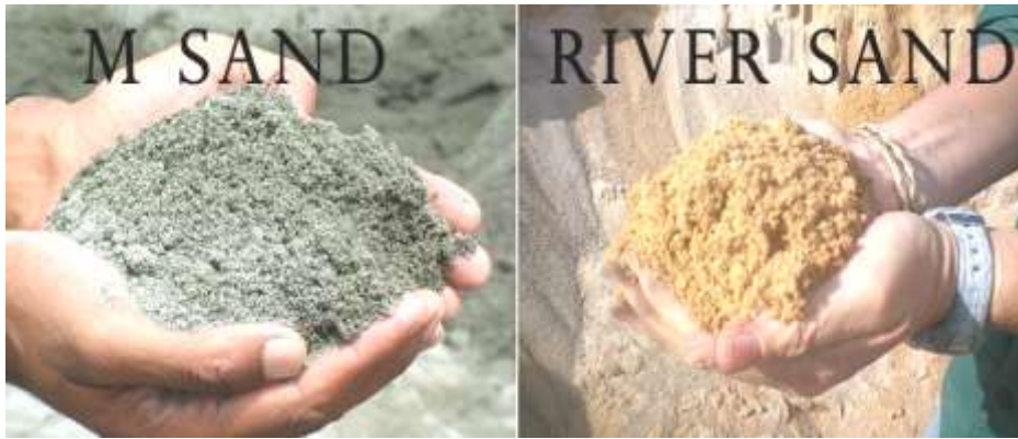
Fig. 1: Image of M-sand and River sand
