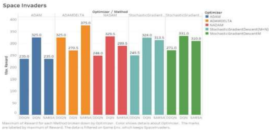
Fig. 8: Maximum rewards obtained after testing the model trained with different methods on another environment (Space Invaders)
